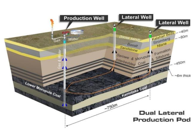
The above schematic provides a visual representation of how Tlou's production pods have been drilled. This is indicative only and not to scale.
