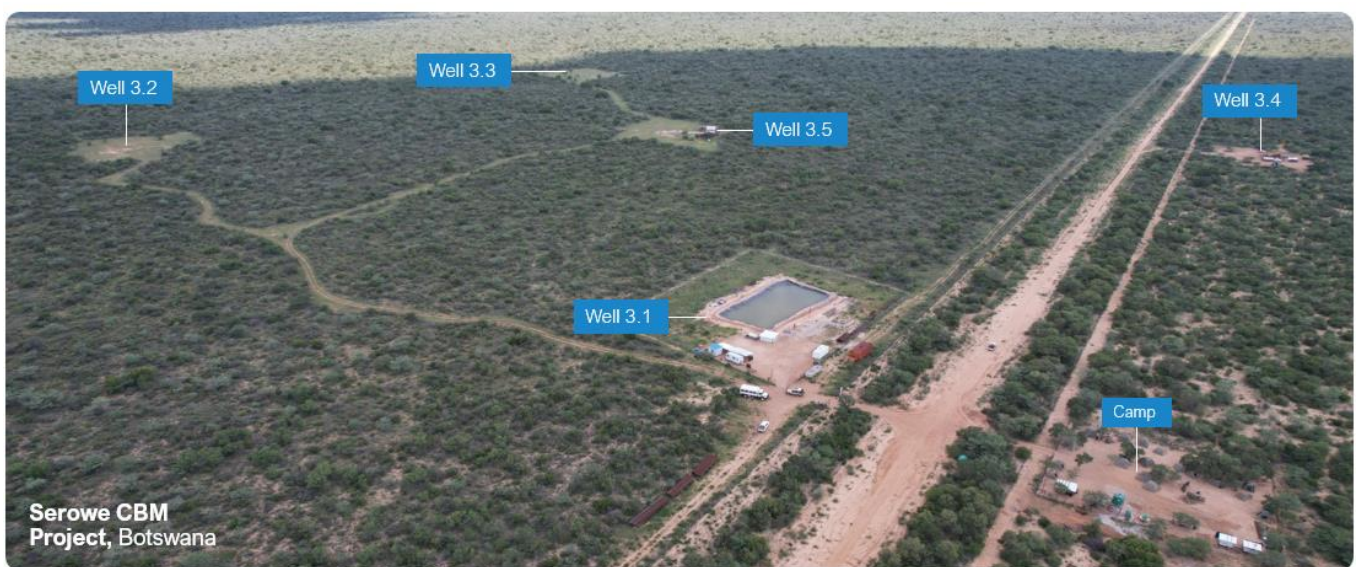
Figure 1. Project Pitse is a five-well pilot cluster which represents the first phase of development at the Serowe CBM Project.
